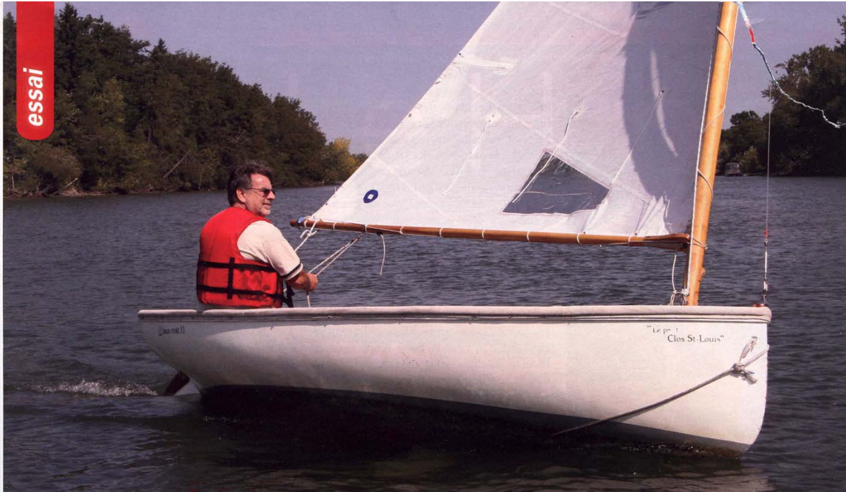
Louis Ducharme sailing upwind aboard his Bras d'Or 11 on the Richelieu River behind Jeannotte Island. Note the textile rubrail designed to absorb shocks when docking.
